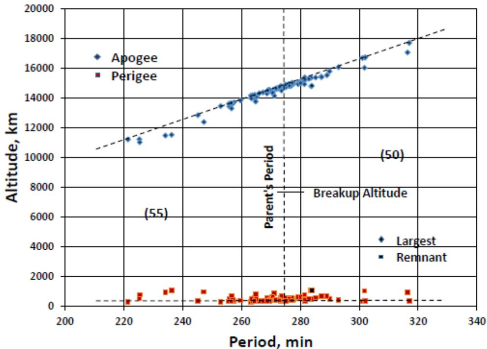
**Fig. 5.** Gabbard diagram of first 106 cataloged fragments of Briz-M rocket (28944).
