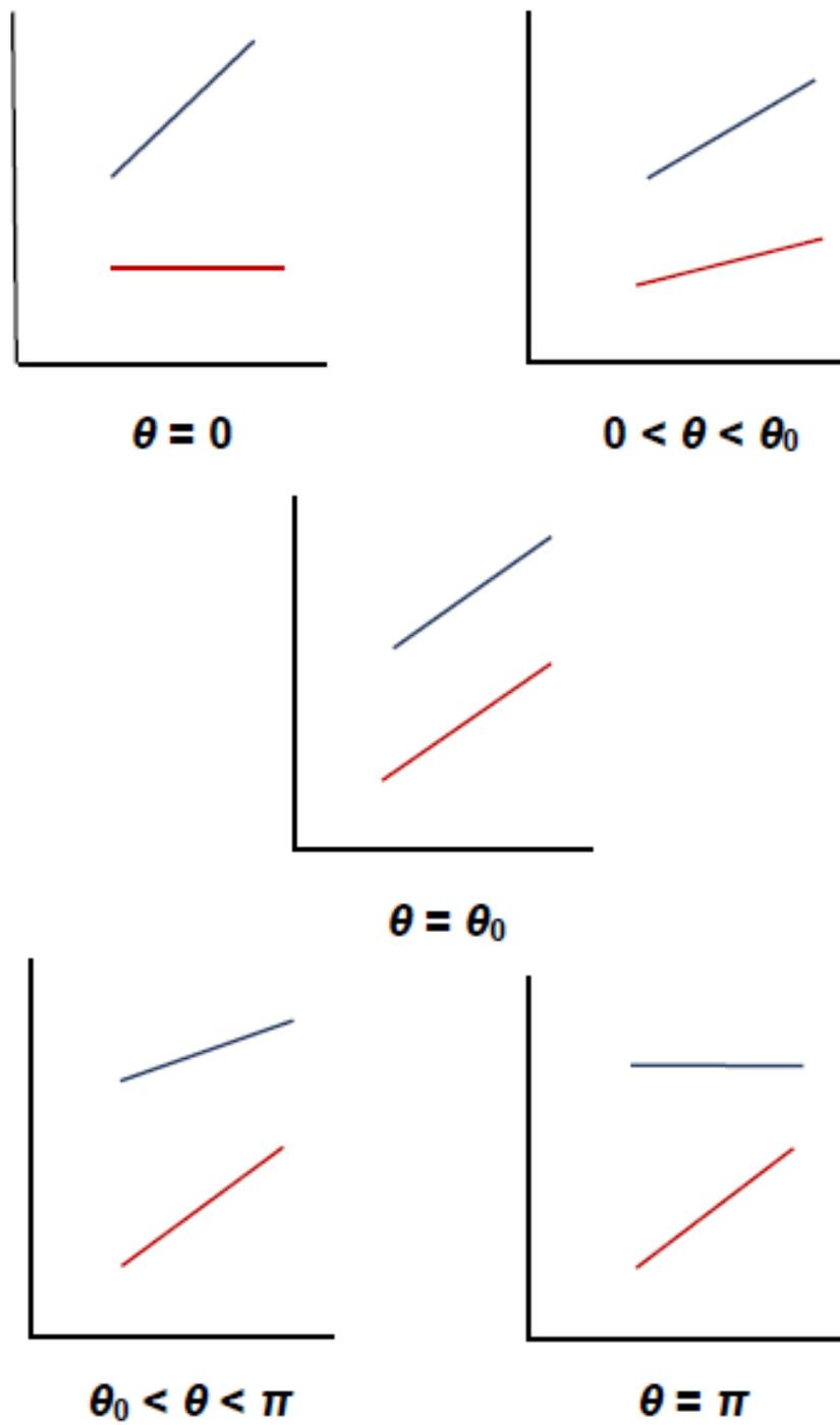
**Fig. 3.** Gabbard Diagrams for various true anomalies of the fragmenting satellite.
