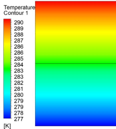
**Figure 5.** Stratification at steady state
