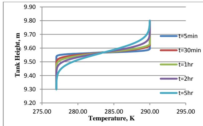
**Figure 6.** Thermocline thickness
