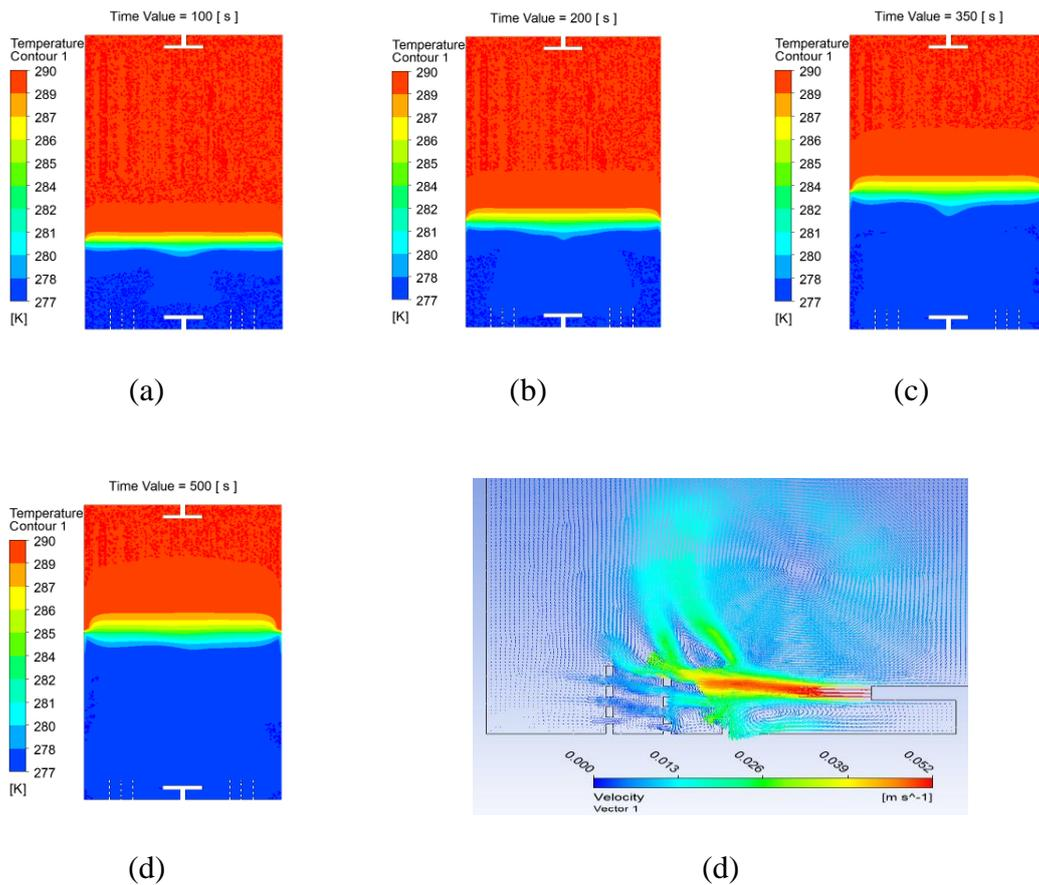
**Figure 7.** Effect of perforated dampers on thermocline
