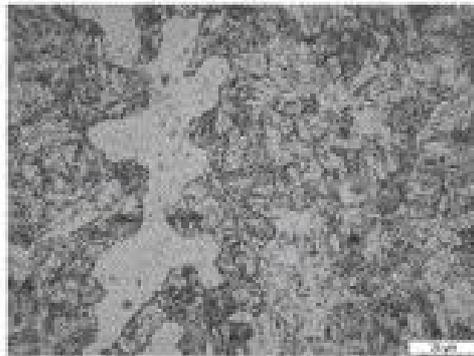
**Fig. 1:** Microstructure of Grade 91 Alloy Steel <sup>[4]</sup>. This photograph appears courtesy of [B. ShashankDutt]
