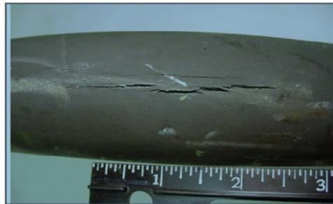
**Fig. 2:** Stress Corrosion Cracking in P91 <sup>[2]</sup>.
