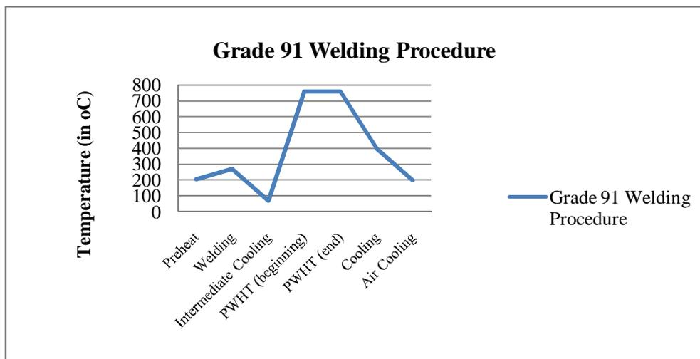
**Fig. 3:** Welding of Grade 91 seamless pipe (P91) summarized at a glance.
