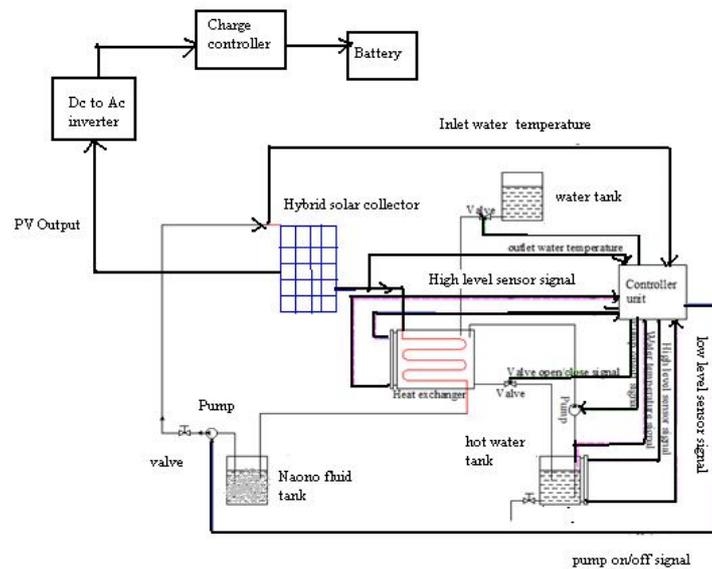
**Fig. 3:** Hybrid solar system for hot water supply and battery charging.
