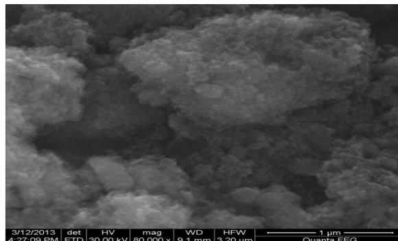
**Fig. 1:** SEM Image of Al<sub>2</sub>O<sub>3</sub>/water (0.5 volume %) Nanofluid before sonication.
