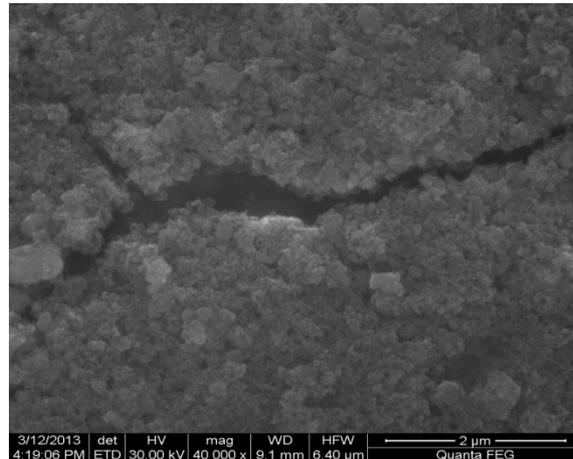
**Fig. 2:** SEM Image of Al<sub>2</sub>O<sub>3</sub>/water (0.5 volume %) Nanofluid after sonication.
