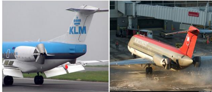
Fig. 1: A KLM with reverse thrust buckets (left) [6] and Northwest DC9's used to pushback with reverse thrust "Power Back"(right). [7]
