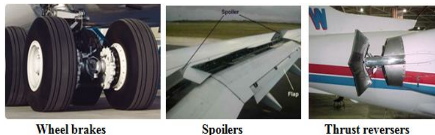
Fig. 2: Different decelerating devices installed on current commercial aircrafts such as wheel brakes, spoilers and thrust reversers.
