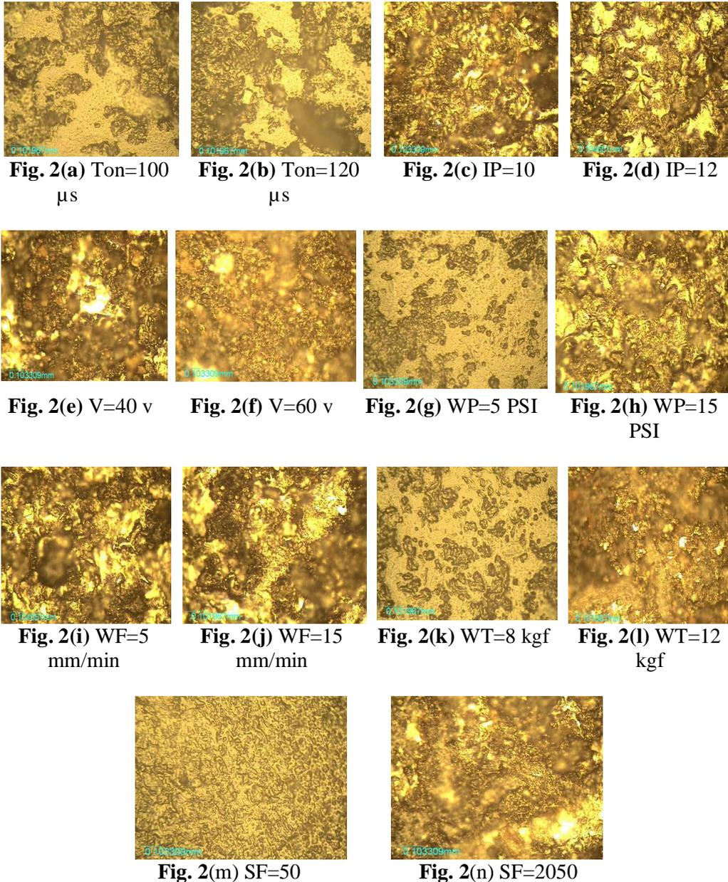
**Fig. 2** (a to n) Surface Topography of WEDM surface of Titanium alloy at different Test Conditions.
