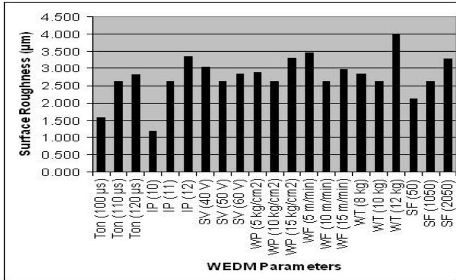
Fig. 1: WEDM parameters vs. Surface Roughness.
