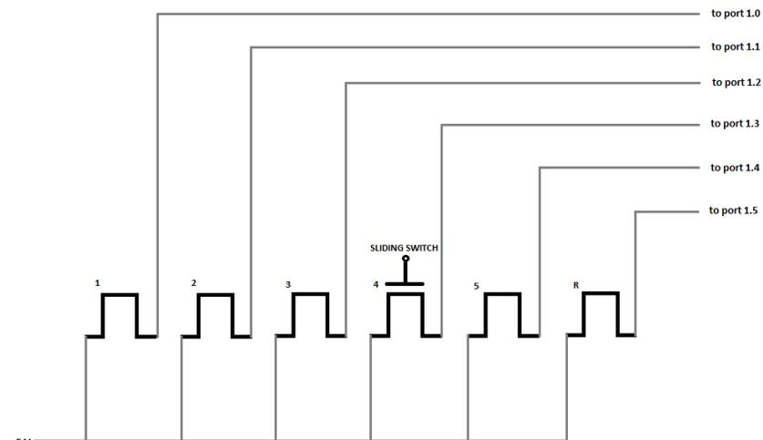
**Fig. 3:** Internal connections of switches in the steering.
