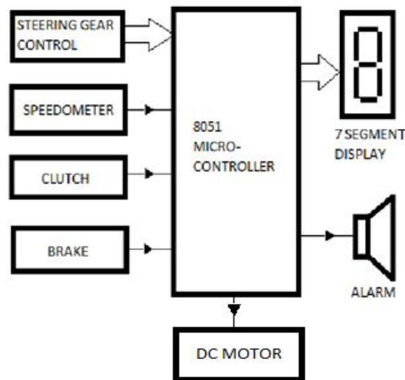
Fig. 1: Block diagram of the stress-less gear system.
