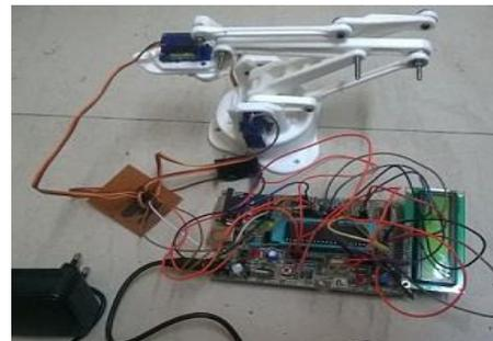
Fig. 4: robot arm with pic board
