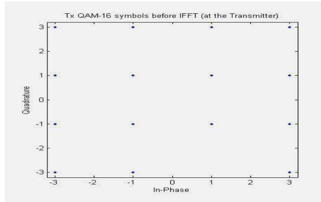
**Figure 5. Successive Results pertain to transmit symbols before IFFT using symbol rate sampling.**
