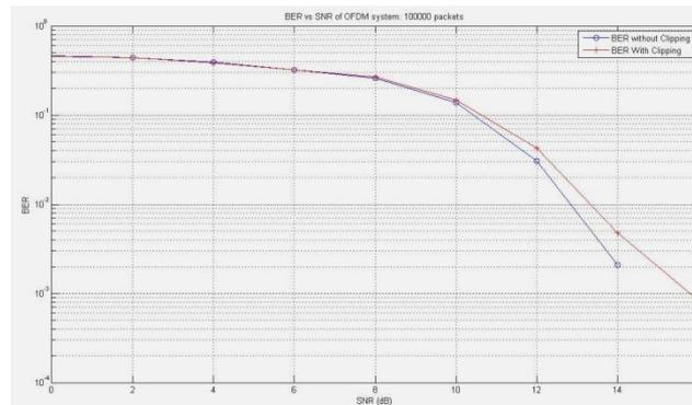
**Figure 11. BER performance with clipping Simulations support the use of the variance of the posterior red colour as an indicator of when the OFDM system in With Clipping BER vs SNR. It is here compared with the actual error in the simulations blue colour .OFDM Without Clipping BER vs SNR**
