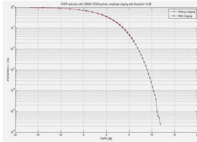
**Figure 9. The performance of OFDM PAPR with Without Reduction Amplitude Clipping.**
