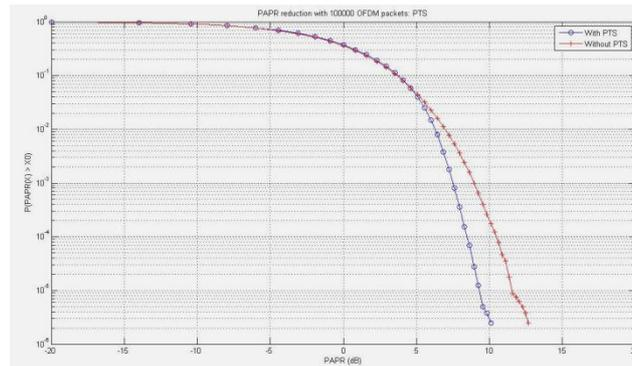
**Figure 10. OFDM PAPR With Without Reduction Partial transmit sequence (PTS) combined**
