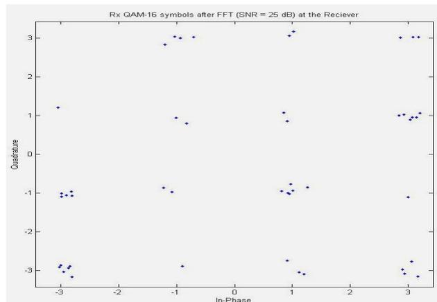
**Figure 6. Successive Results pertain to receiver symbols after FFT using symbol rate sampling.**
