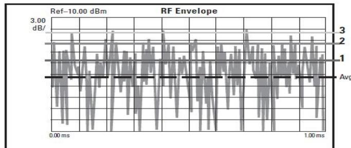
**Figure 1A: construction of a CCDF curve**
