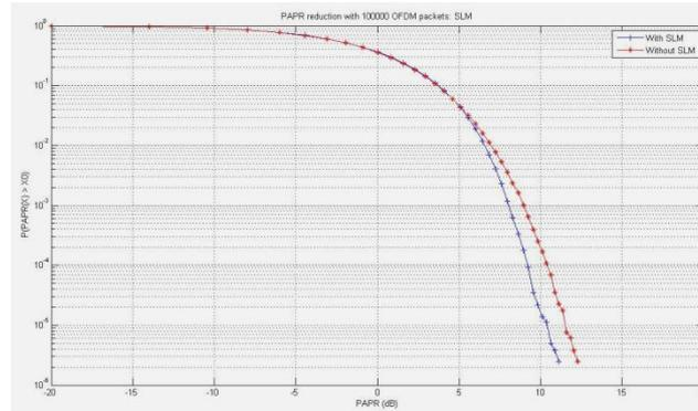
**Figure 12. OFDM PAPR With Without Reduction Partial Transmit Sequence (SLM)**
