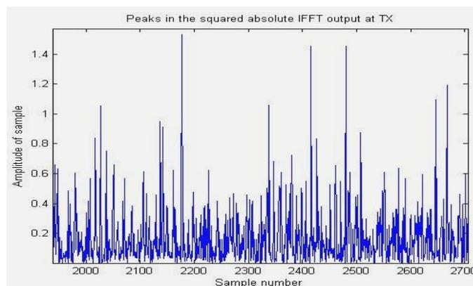
**Figure 7. Successive peak Results pertain to Squared Absolute transmit symbols after IFFT showing peaks without PAPR suppression**
