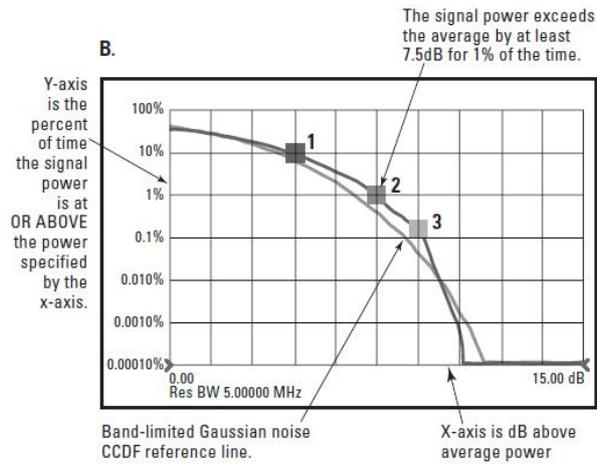
**Figure 1B: CCDF curve of a typical OFDM signal**
