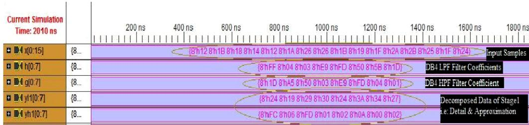
**Figure 2:** Synthesis waveform for I stage decomposition
