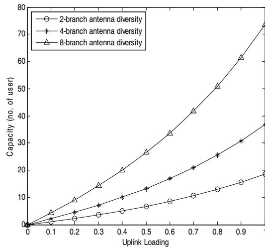
**Figure 6:** Effect of antenna Diversity on WCDMA capacity with  $\beta=0.7$  &  $i=0.6$  for 144kbps data rate applications.
