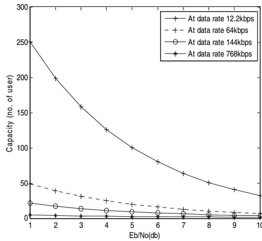
**Figure 1:** Effect of high data rate services on WCDMA capacity.
