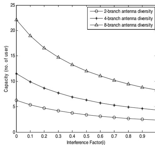
**Figure 9:** Effect of antenna Diversity on WCDMA capacity with  $\beta=0.4$  & 100% loading for 768kbps data rate applications.
