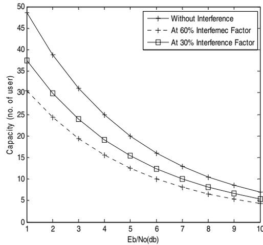
**Figure 3:** Effect of Interference on WCDMA capacity for video services.
