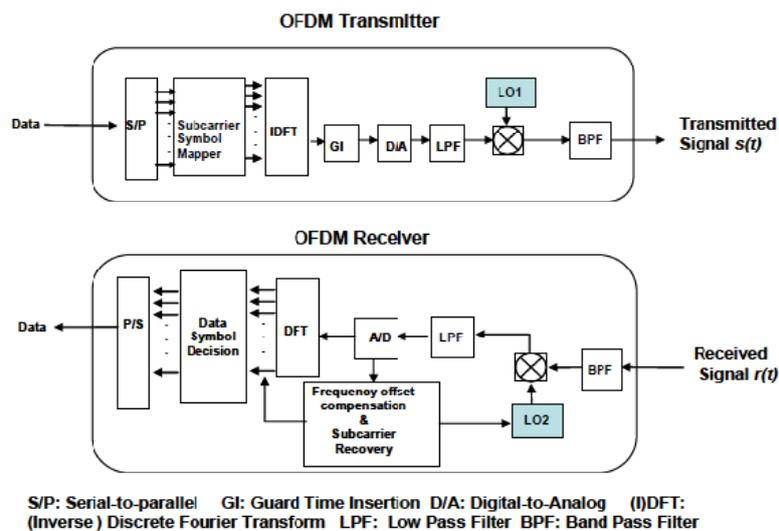
**Figure 2:** Conceptual diagram for the OFDM transmitter and receiver.
