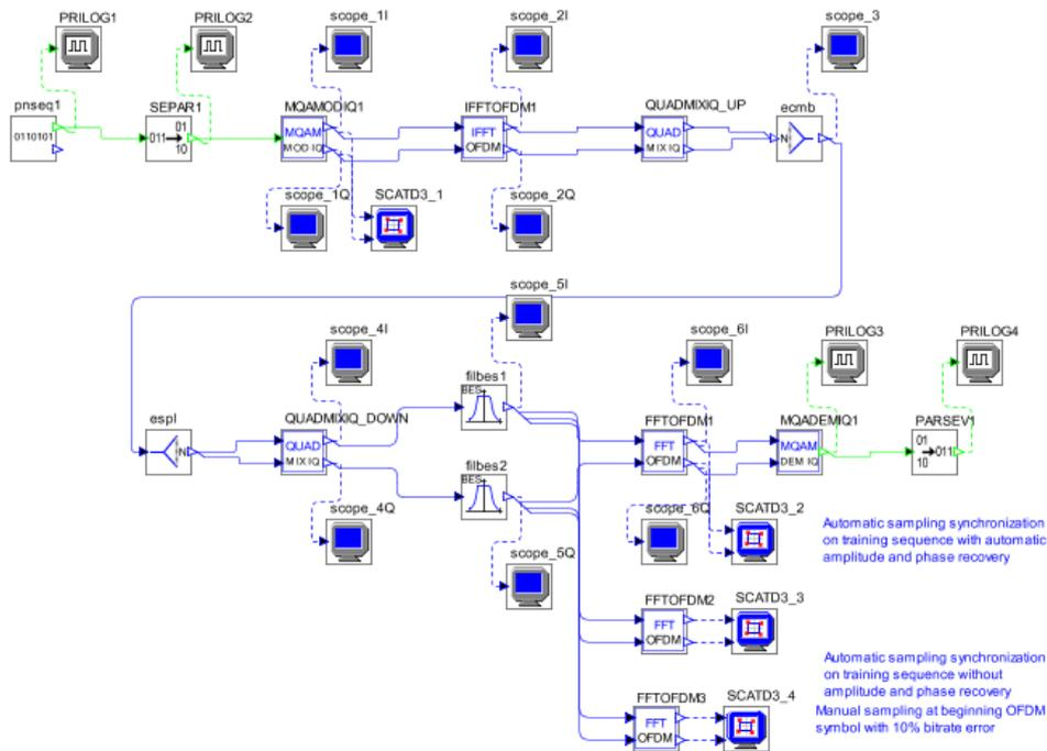
**Figure 3:** Simulation set-up.
