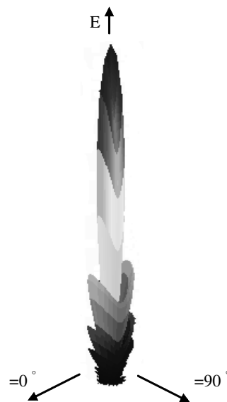
Figure 3: 3D Radiation pattern of circular array of Nylon rod antennas.
