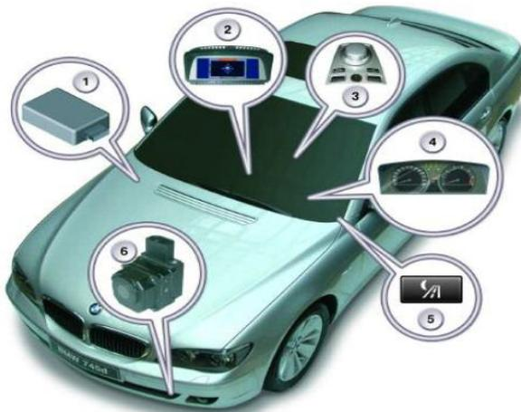
**Fig. 2:** Component of night vision system.
