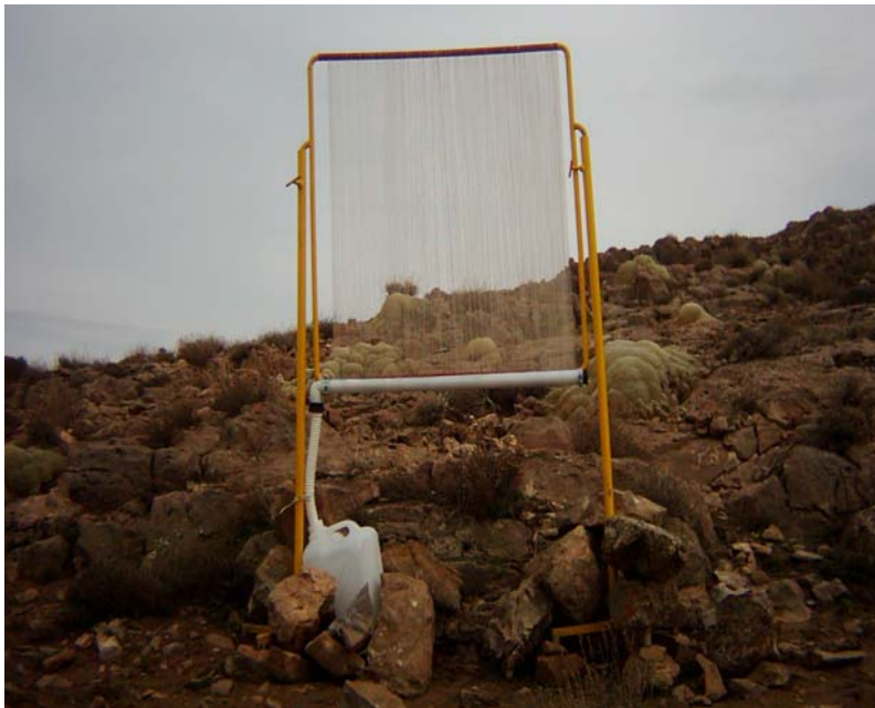
Figure 4 : Flat rectangular fog collector
