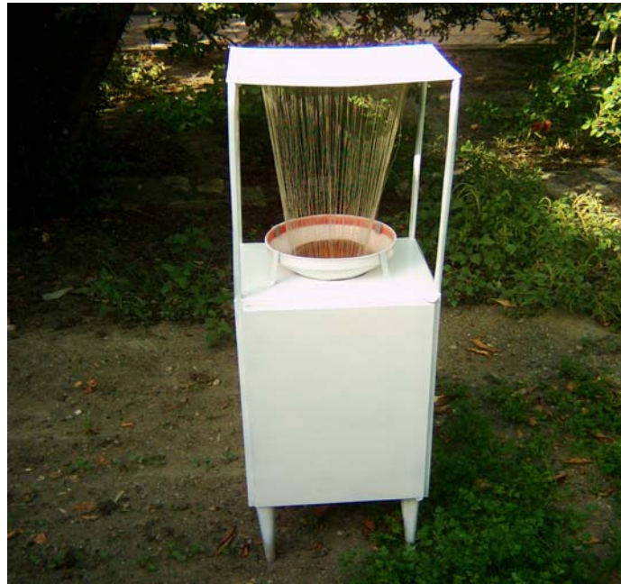
Figure 5 : Simple cylinder fog collector
