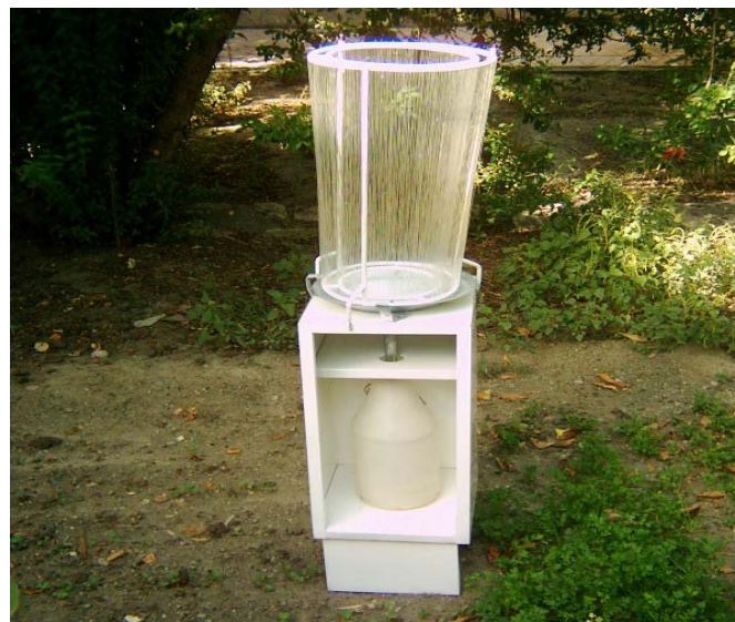
Figure 6 : Double cylinder fog collector
