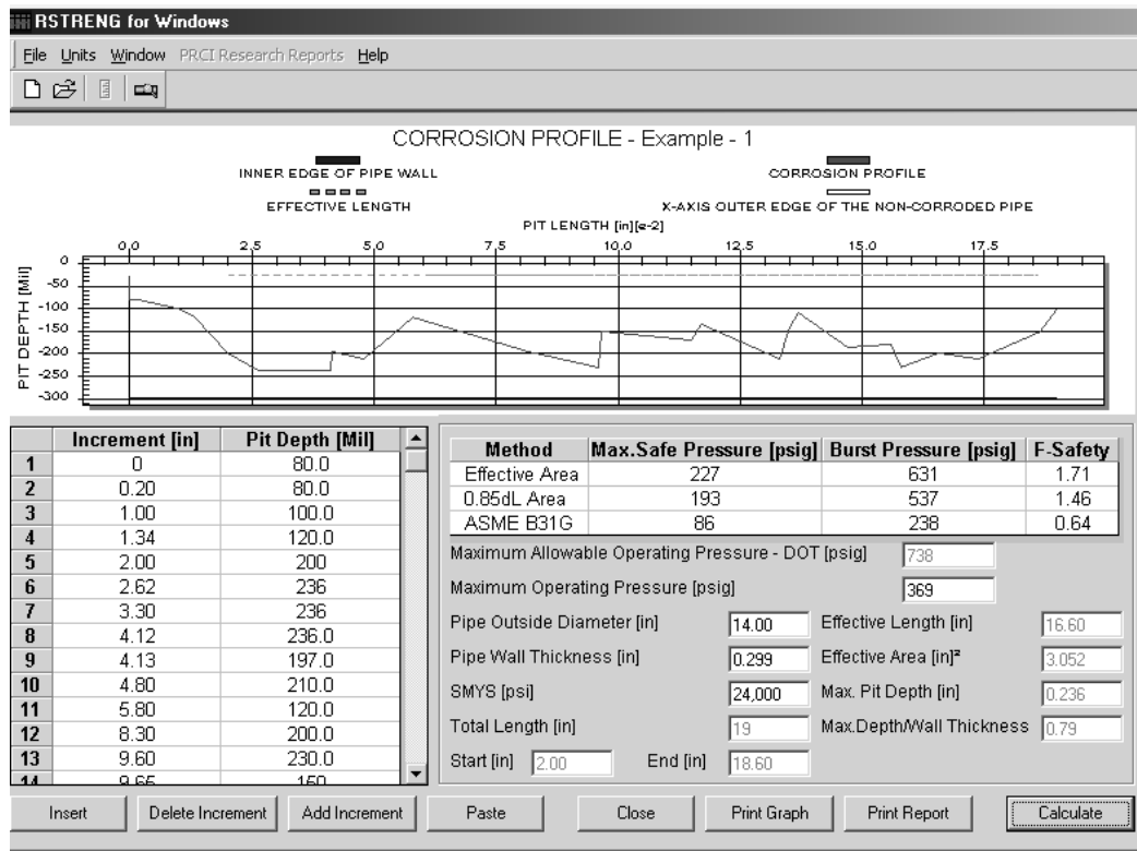
Figure 8a: If the minimum yield strength was not determined from the destructive tension tests or from the nondestructive ABI tests; the maximum safe pressure would only be 86 psi (because of the CFR conservative value of 24,000 psi for the yield strength for undocumented pipeline instead of the minimum ABI-measured value of 40,200 psi) which is below the current operating pressure of 100 psi (7 kg/mm 2 ) instead of the 143 psi of Fig. 7
