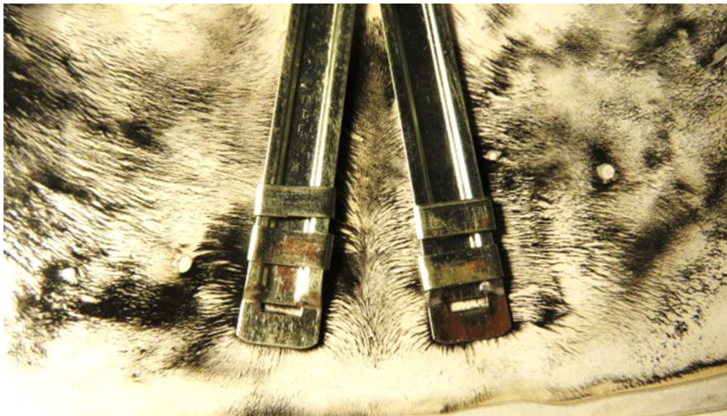
Figure 2 . The magnetic field lines of two arms with the same polarities. They repel each other and give an inverted 'V' shape as shown. (Dimensions of each arm: 8 cm long, weight 2.9 gm, 1.3 cm wide and 0.033 cm thickness)
