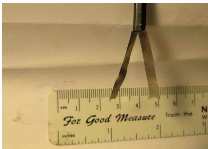
Figure 4(B): Two Ni pieces of the same magnetic charges, form an inverted "V" shape, due to the repulsive forces. (Dimensions of the Ni pieces: 4.0 cm long, weight 0.15 gm.) (The magnetic field lines are similar to those of figure 2).
