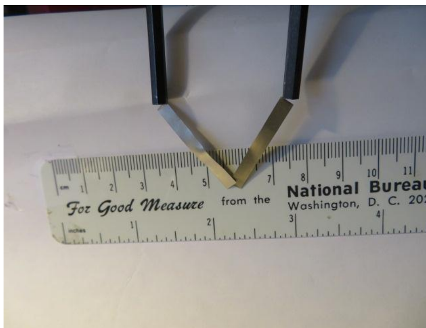
Figure 4(A): Two Ni pieces of opposite magnetic charges, form a 'V' shape, due to the attractive forces between them. (Dimensions of the Ni pieces: 3.1 cm long, weight 0.11 gm; All four pieces, including in Figure 4(B) having thickness of 0.01016 cm, and a width of 0.4 cm). (The magnetic field lines are similar to those of Figure 3).
