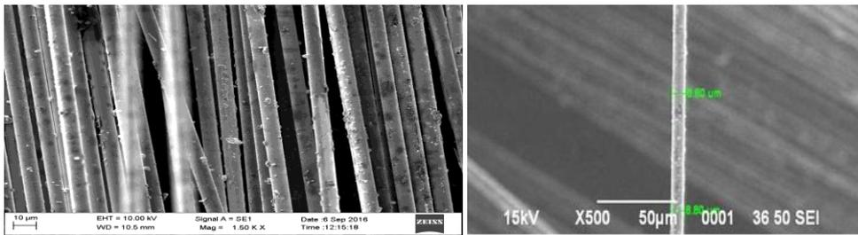
**Figure (2) a & b.** Nickel coated carbon fibre
