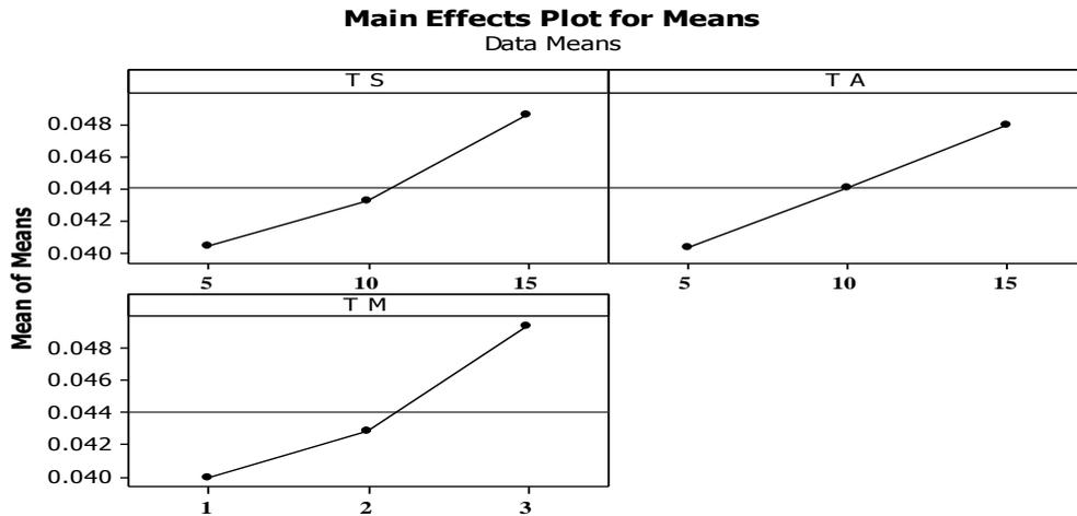
**Figure1.** Mean effect plot for means for thickness of coating on fiber
