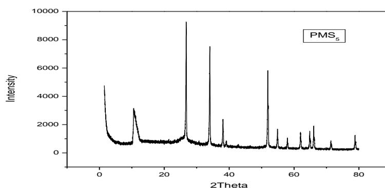
**Figure 2:** shows X-ray diffraction pattern of Polyaniline/MgSnO<sub>3</sub> (50 wt %)
