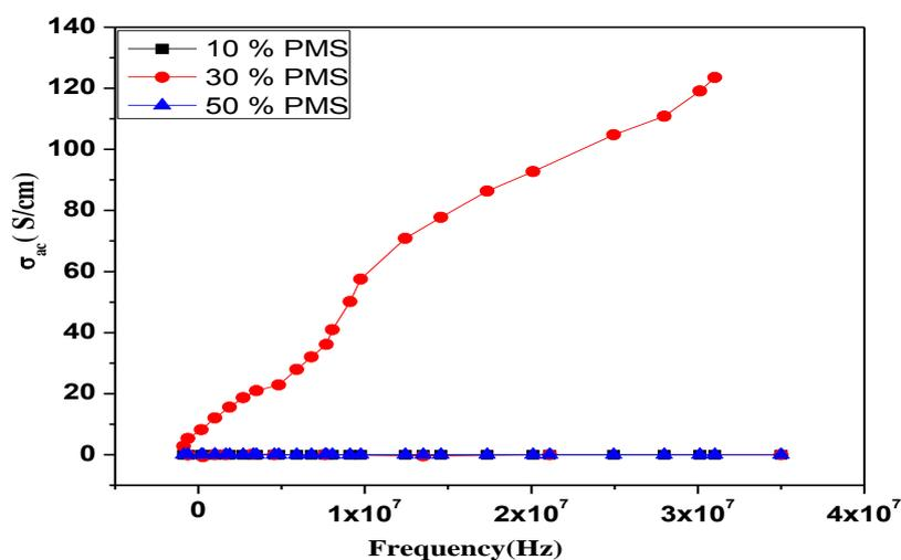
**Figure 8:** Variation of ac conductivity as a function of frequency for Polyaniline MgSnO<sub>3</sub> Composites
