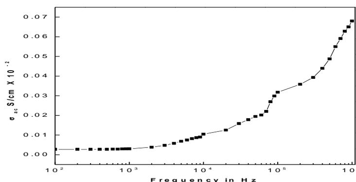
**Figure 7:** Variation of ac conductivity as a function of frequency for polyaniline
