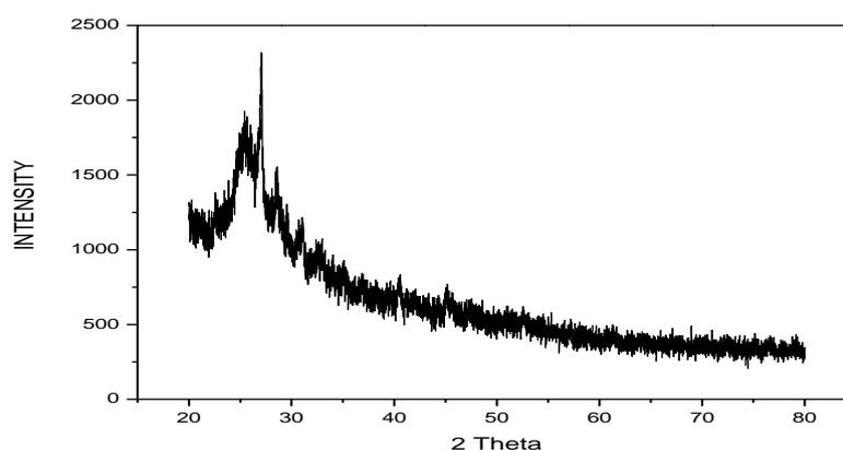
**Figure 1:** Shows X-ray diffraction pattern of Polyaniline
