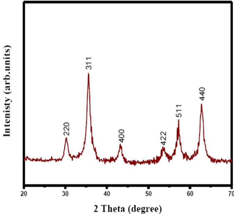
**Fig.1.** X-ray Diffraction Analysis of  $Fe_3O_4$ /Activated Carbon Nano composite
