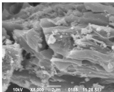
**Fig.3.** Scanning electron microscopy of Fe<sub>3</sub>O<sub>4</sub>/Activated Carbon Nano composite
