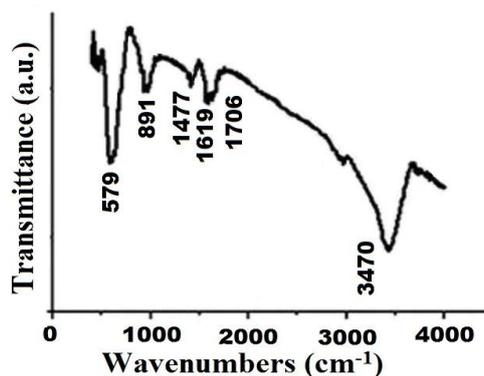
**Fig.2.** Fourier Transform Infrared Spectroscopy of Fe<sub>3</sub>O<sub>4</sub>/Activated Carbon Nano composite
