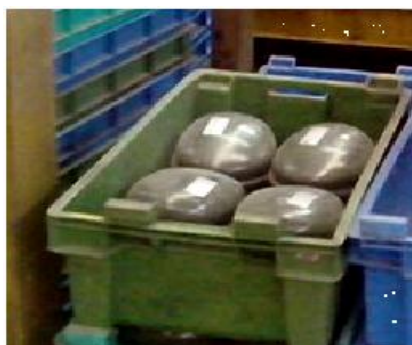
Fig.1: Orientation of compressors in bin
