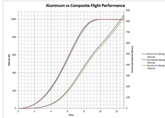
**Fig. 5.** Aluminum vs composite casing flight performance
