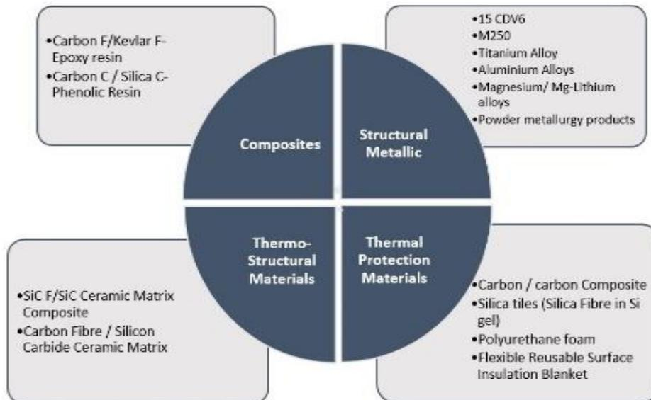
Fig. 4. Classification materials in SRM casing
