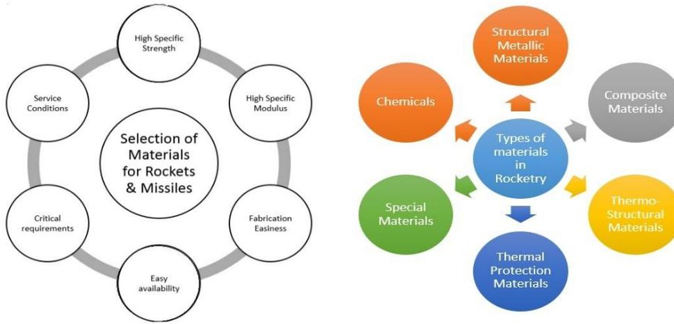
Fig. 3. Selection of Materials and Types of materials used in Rocketry
