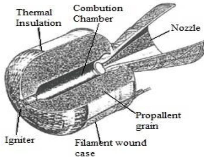
**Fig. 1.** Solid Rocket Motor
