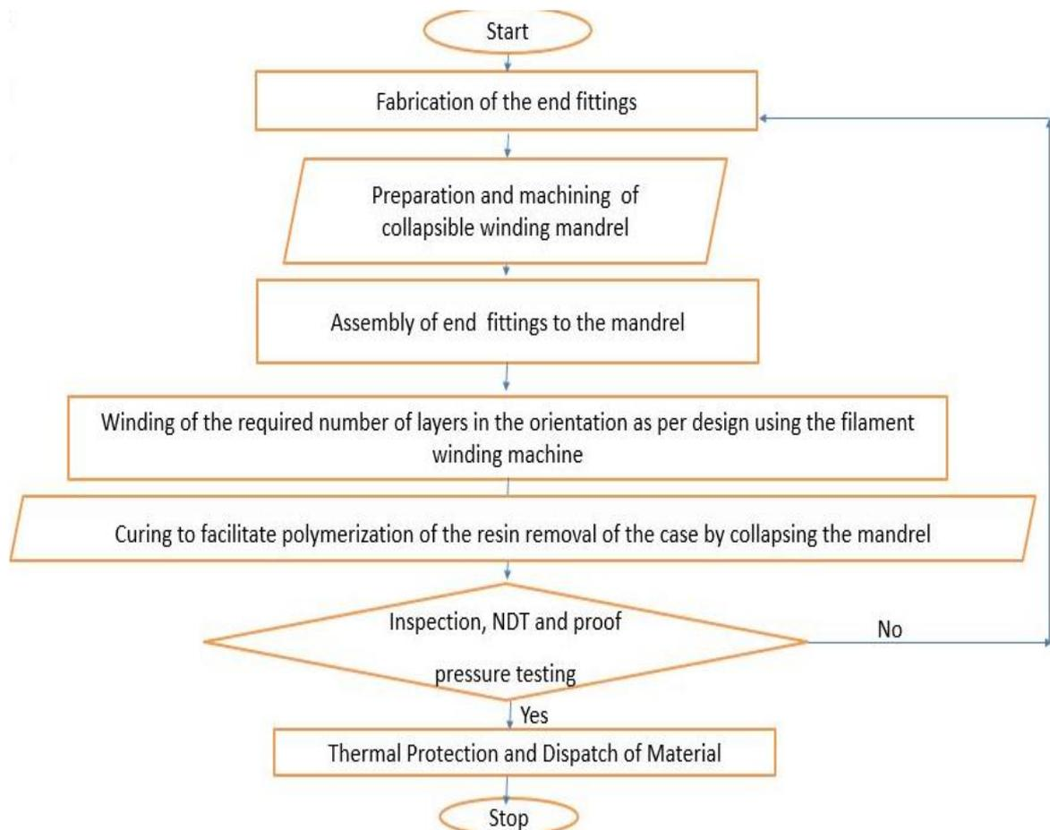
**Fig. 6.** Flow chart showing the steps in fabrication of composite casing
