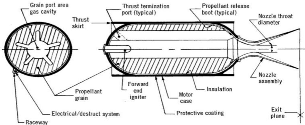
**Fig. 2.** Components of Solid Rocket Rocket Motor (SRM)
