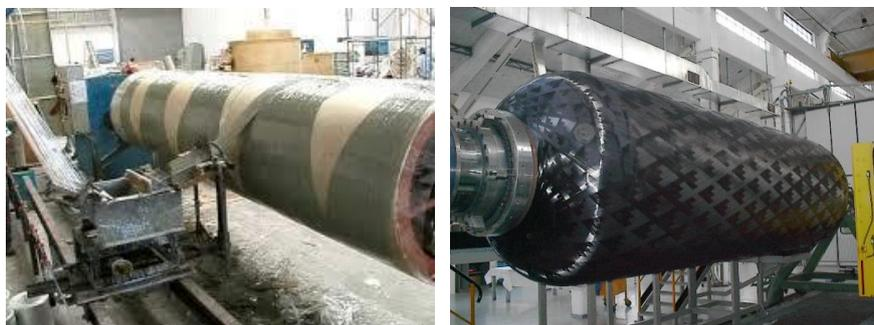
Fig. 8. Filament case manufacturing over drum and mandrel
