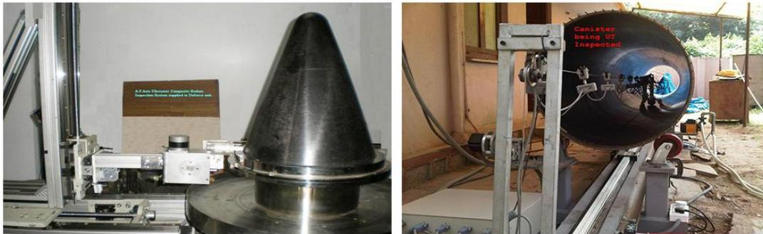
**Fig. 9.** NDT Inspection of casings
