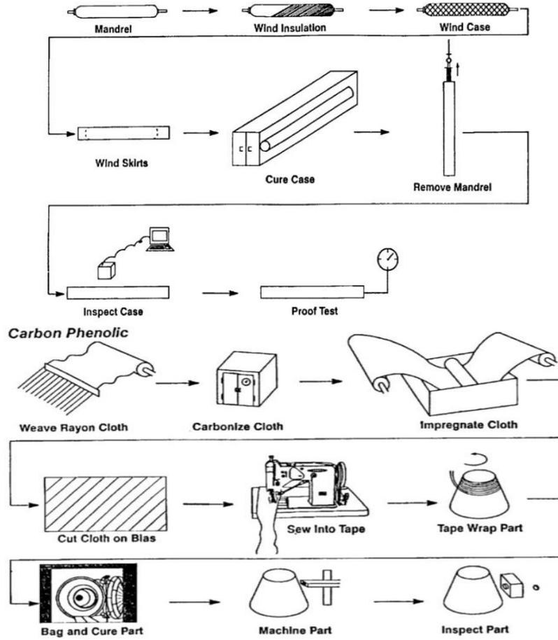
Fig. 7. Filament wound case and Nozzle manufacturing process steps
