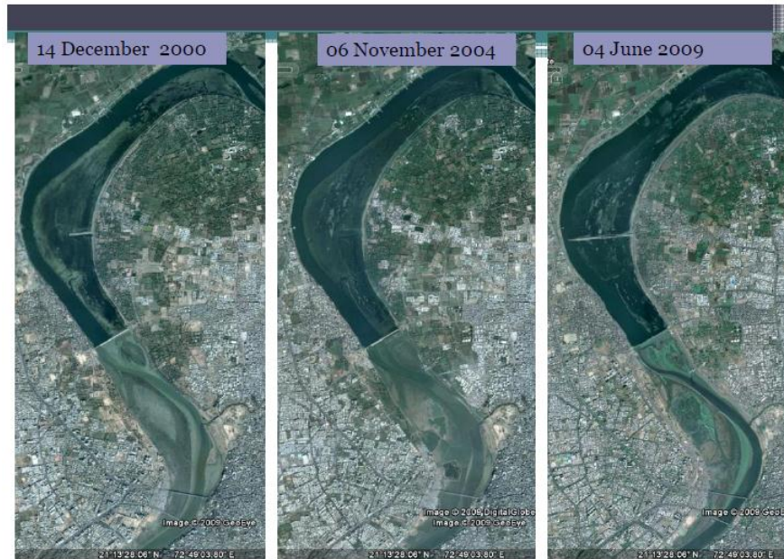
Shift in River Tapi and storage of water at weir cum cause way, hence shrinkage of river downstream due to siltation.
