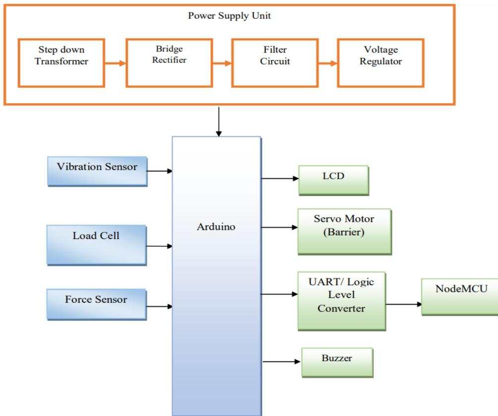
**Fig 4.1** Block Diagram
