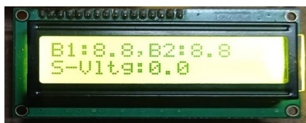
Figure 5: Voltage across Batteries and Solar Panel.
