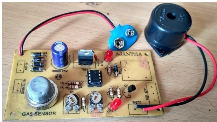
Figure 1: LPG leakage detection and alert system
