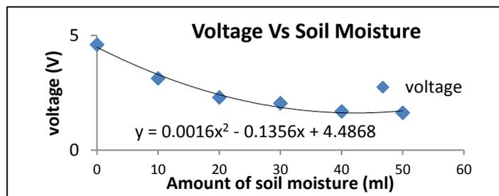
**Figure 3:** Sensitivity graph for Soil Moisture Sensor
