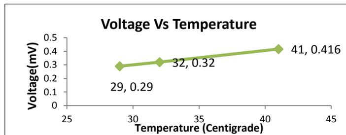
**Figure 2:** Sensitivity graph for Temperature Sensor
