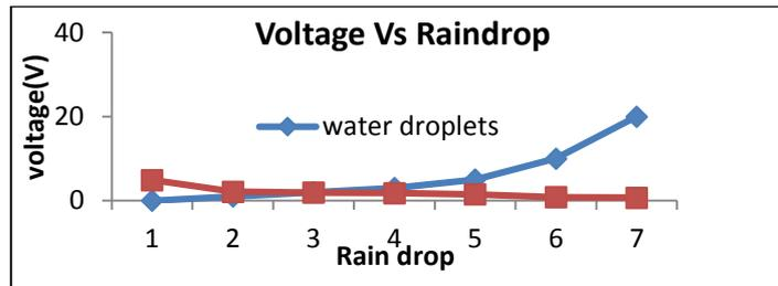
**Figure 4:** Sensitivity graph for Raindrop Sensor
