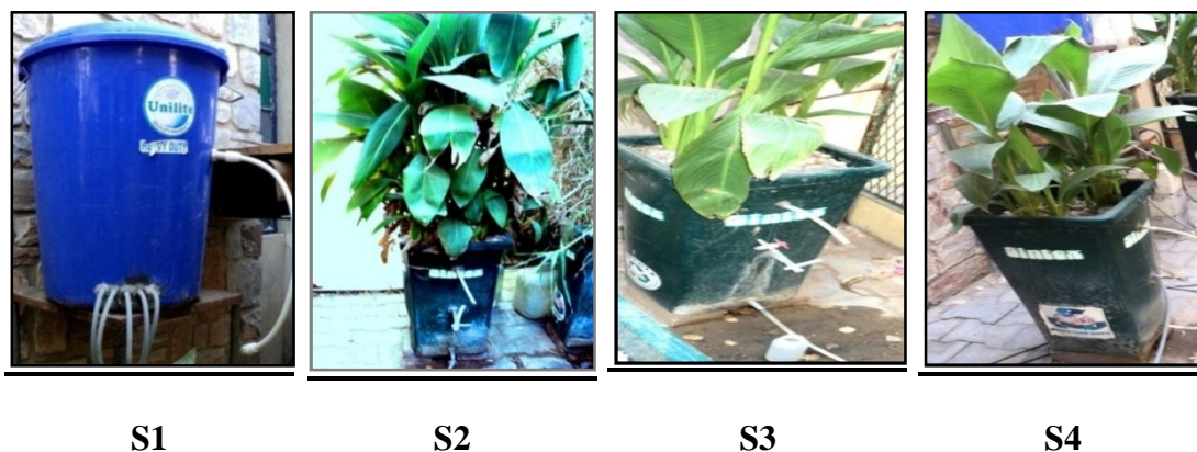
Fig. 2: Storage tank; S1, S2, S3 planted with Canna indica but had different gradation of media.
