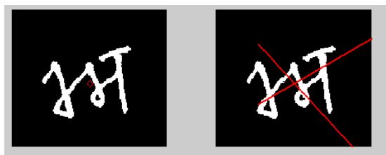
Figure 2: (a) Find center of the image (b) Visualization of a projection of angle 45^\circ
