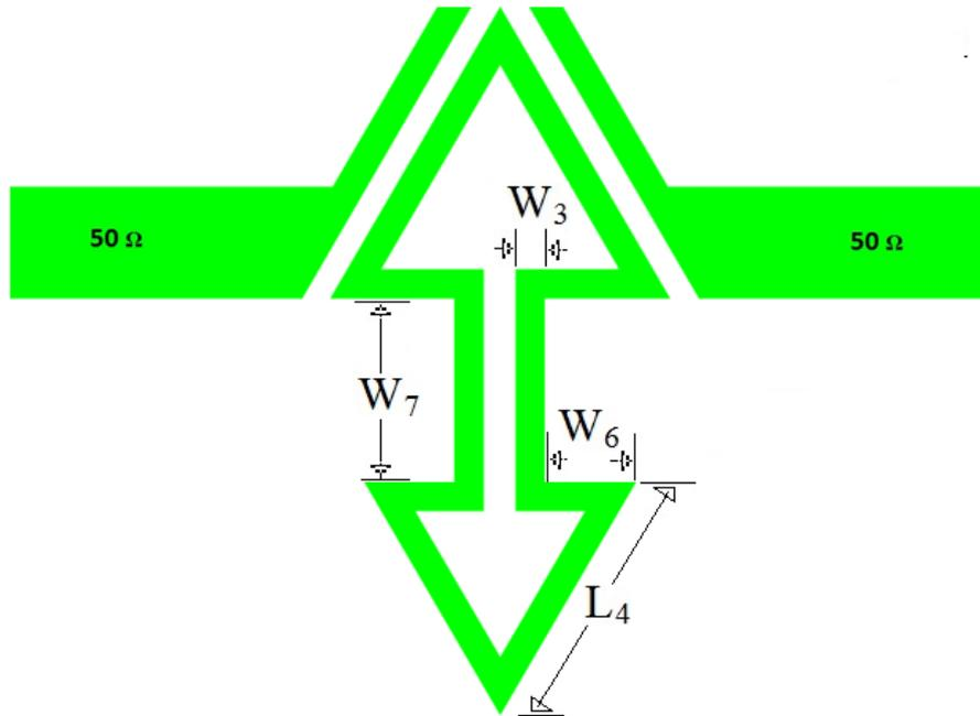
**Figure3.** Structure of the proposed Filter.
