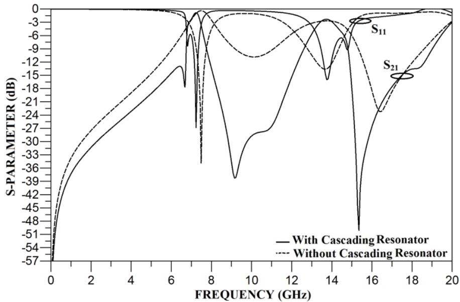
**Figure 4.** Frequency response of with and without cascaded open loop triangular ring resonator.
