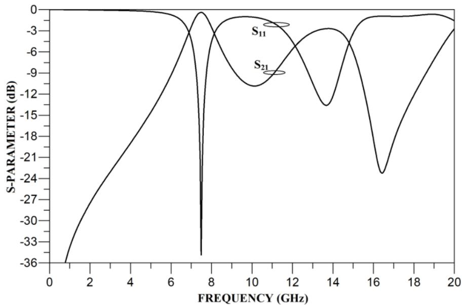
**Figure 2.** Frequency response of open loop triangular ring resonator coupled in series with transmission line with loaded stub.
