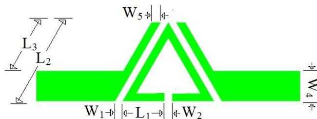
**Figure 1.** Structure of open loop triangular ring resonator coupled in series with transmission line with loaded stub.
