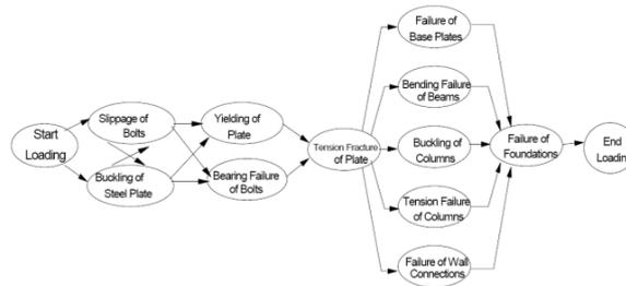
Fig. 3.1: Failure modes of steel plate shear wall.
