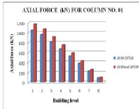
Figure 3.9: Axial force in (kN) for column no.1
