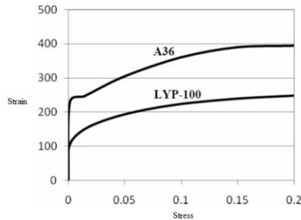
**Fig. 2.1:** Stress strain curve of A36 and LYP-100 steel.
