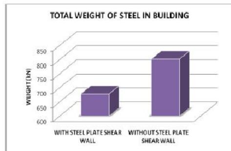
**Figure 3.14:** Total weight of steel in (KN).
