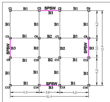
**Figure 2.2:** Plan of G+6 storey steel building with SPSW
