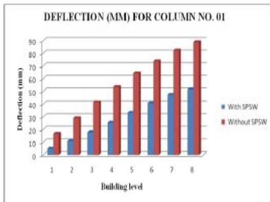
Fig 3.2: Deflection in (mm) for column no.1
