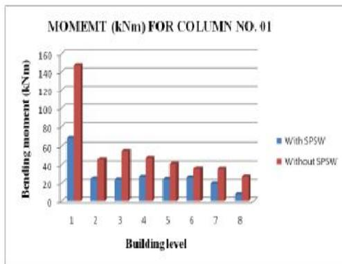
Figure 3.8: Bending moment for column no.1
