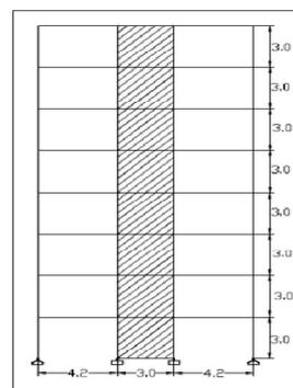
**Figure 2.3:** Elevation of G+6 storey steel building with SPSW
