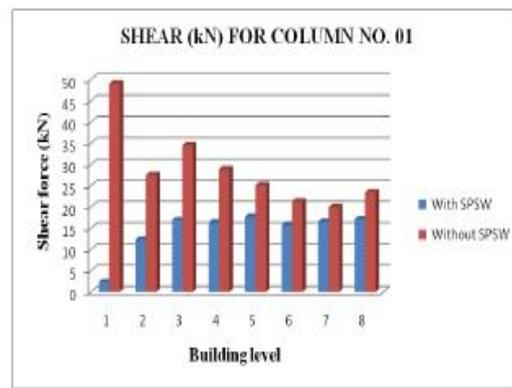
Fig 3.3: Shear force in (kN) for column no.1
