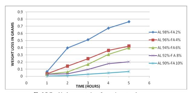
Fig 1.8 Graphical representation of corrosion rate values
