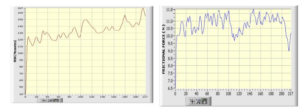
Fig 1.6 Wear vs Distance for 30N load Fig 1.7 Friction vs Distance for 30N load
