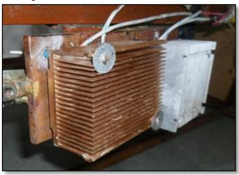
Figure 9: TEG Setup fabricated for present study
