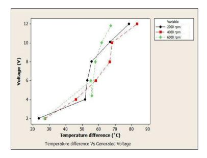
Figure 12: Shows that temperature difference is directly proportional to voltage
