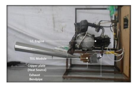
Figure 10: Experimental setup of present study
