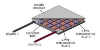
**Figure 2:** Thermoelectric generator [4]
