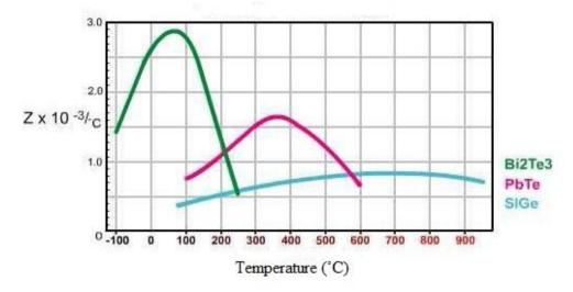
**Figure 3:** Performance of Thermoelectric Materials at various temperatures [4]
