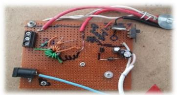
Figure 7: Joule Thief Converter (Booster circuit) used in present study
