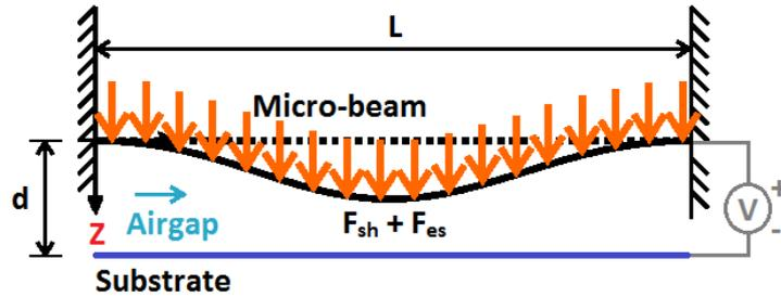
**Figure 1. A schematic view of an electrostatically actuated clamped-clamped micro-beam.**
