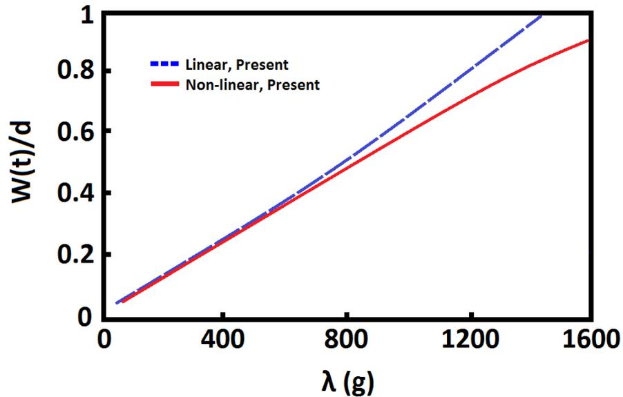
**Figure 4. Linear and non-linear ratio of mid-point deflection of micro-beam calculated for  $T=1$  ms.**
