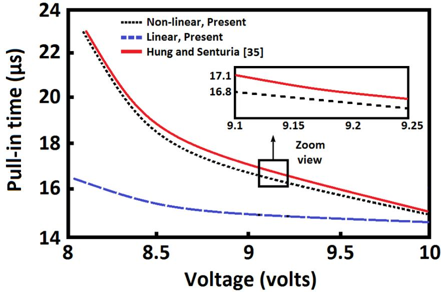
**Figure 3. Pull-in time under electrostatic extinction and mechanical shock.**
