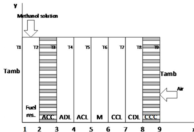
Fig 1: Schematic diagram of passive DMFC
