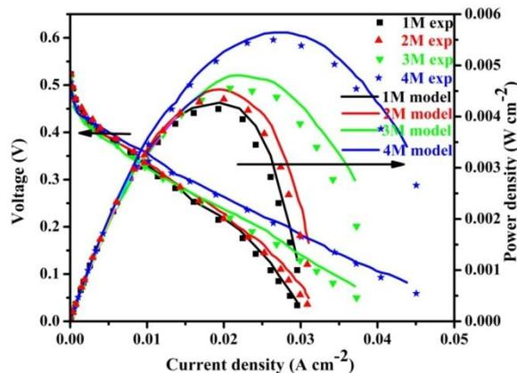
Fig. 2: Comparison of polarization curve and power density curve for different methanol concentrations
