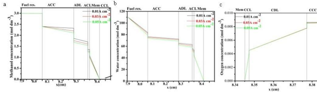
Fig. 3: (a) methanol concentration profile under; (b) water concentration profile; and (c) oxygen concentration profile under 3 m methanol concentrations at current densities of 0.01, 0.03 and 0.05  $\text{A cm}^{-2}$ .
