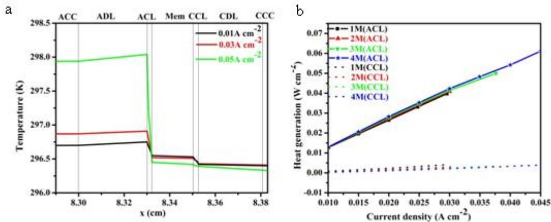
Fig. 4: (a) Temperature profile across the entire passive DMFC for different current densities at 3m concentration.(b) heat generation at ACL and CCL with respect to current density for different methanol concentration.
