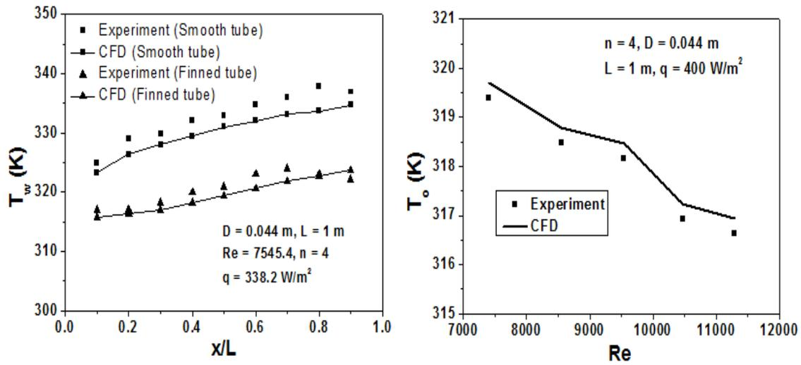
Fig. 4 Comparison between smooth tube and finned tube
