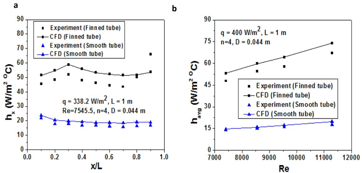
Fig. 5 Comparison between smooth tube and finned tube
