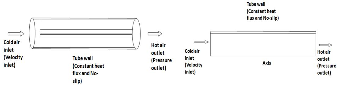
**Fig. 2 Schematic diagram of computational domain and the boundary condition applied to it (a) finned tube; (b) un-finned tube**
