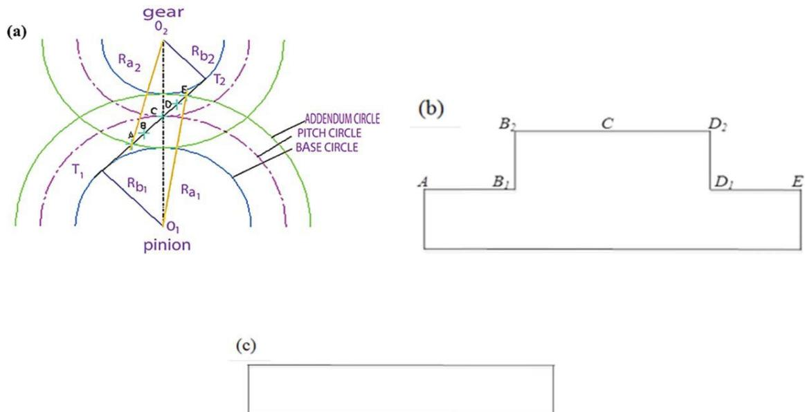
Fig. 1— (a) Path of contact (b) & (c) load distribution for different contact ratio
