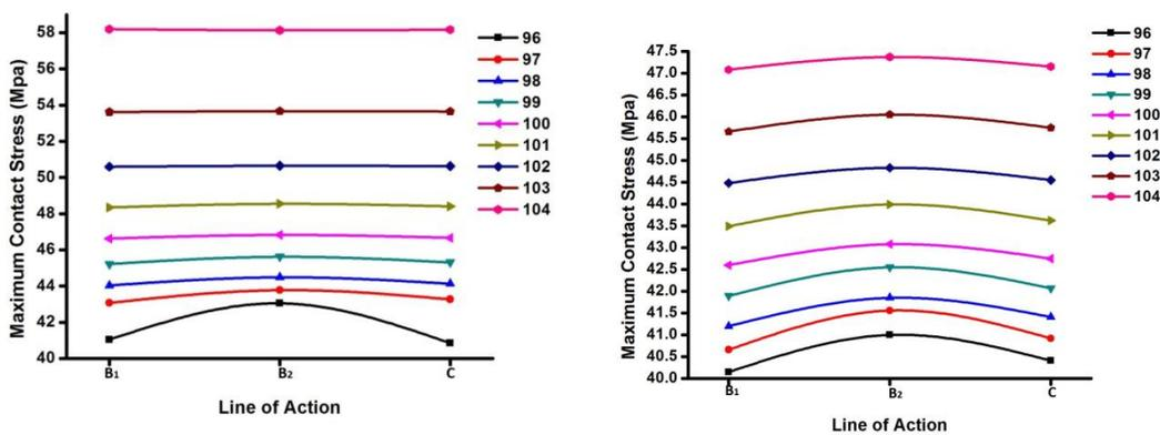
Fig 2: Contact stress on path of contact for pressure angle  $20^\circ$ (a) and  $25^\circ$ (b)
