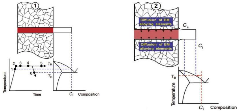
Fig.1.2 Dissolution stage in TLP bonding [3]
