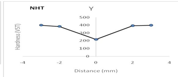
**Fig.4.4 Non Heat Treated Hardness Graph**
