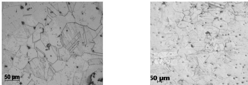
**Fig.4.1 Microstructure of Base Metal of IN718**
