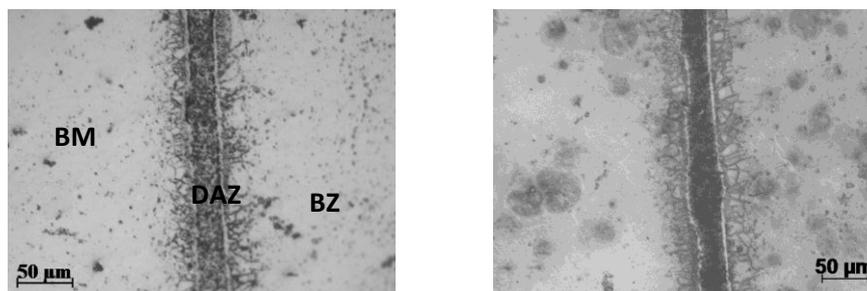
**Fig. 4.2 microstructures of TLP bonded IN718**
