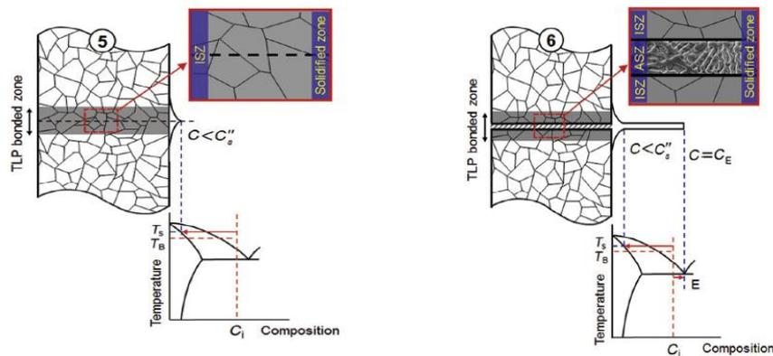
**Fig.1.4 (a) Solid state homogenization**
