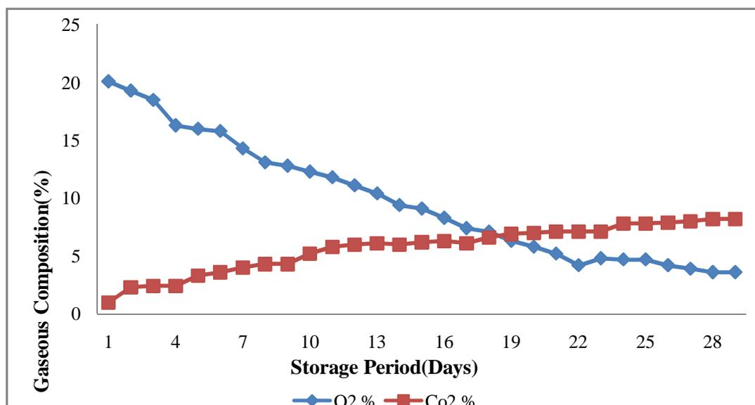
Figure 1: Progression of O<sub>2</sub> and CO<sub>2</sub> concentration of 5kg sample at 8°C with 25cm length diffusion channel.
