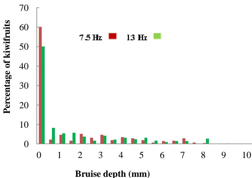
**Figure 2:** The effect of frequency on bruise depth of kiwifruits in vibration acceleration of 0.3 g.
