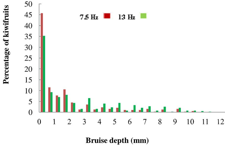
**Figure 3:** The effect of frequency on bruise depth of kiwifruits in vibration acceleration of 0.7 g.
