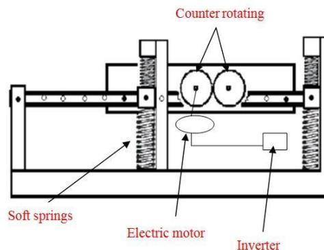
**Figure 1:** Vibration simulator.
