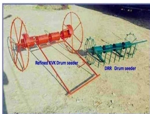
**Figure 1:** DRR drum seeder and Modified drum seeder by KVK.
