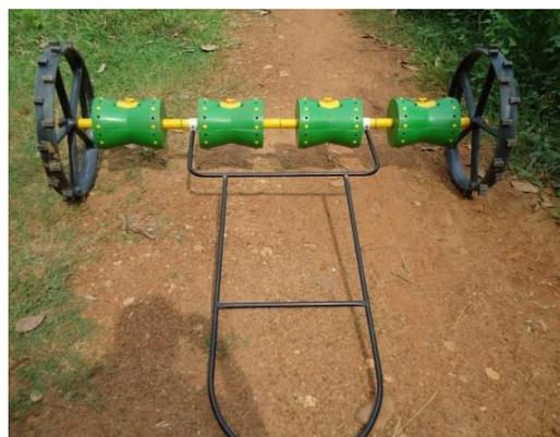
**Figure 2:** TNAU Drum Seeder.
