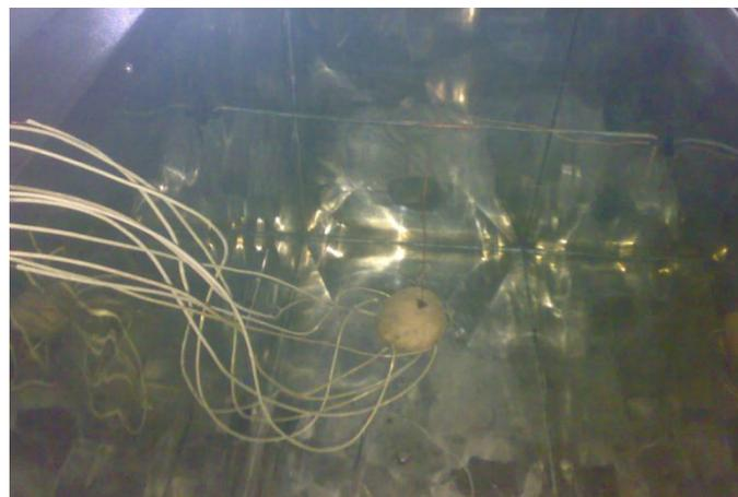
**Figure 2:** Laboratory view of sample (potato) in deep freezer with thermocouples inserted in radial directions.
