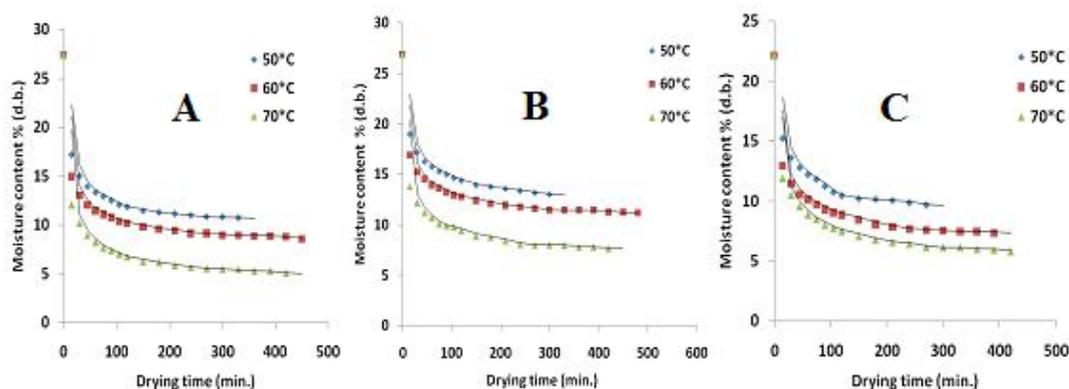
**Figure 2:** Drying curves for Gum kondagogu (*Cochlospermum gossypium*) grade-I (A), grade-II (B), grade-III (C) at temperature 50-70°C in hot air cabinet dryer.
