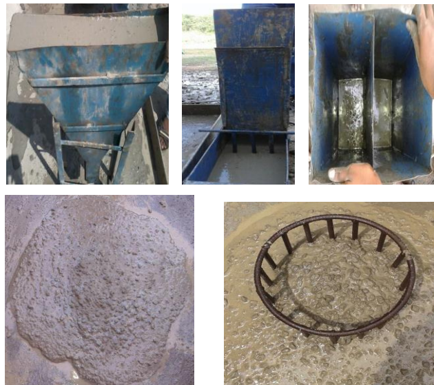
Fig 4. Fresh Properties of SCC: J Ring, V Funnel, L box, U box_and Slump flow
