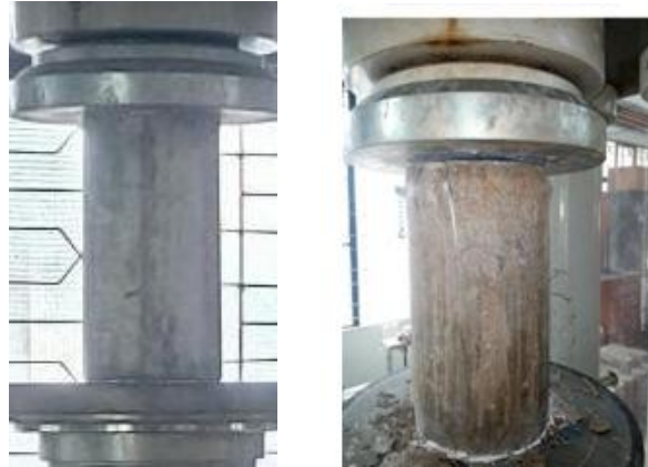
Fig 7. Testing of stub columns in electronic UTM (1000 KN)
