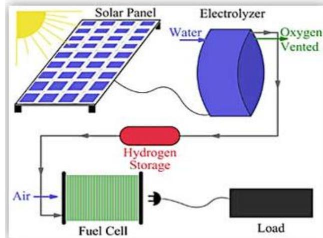
**Figure 2:** The schematic diagram of the solar hydrogen fuel cell system.
