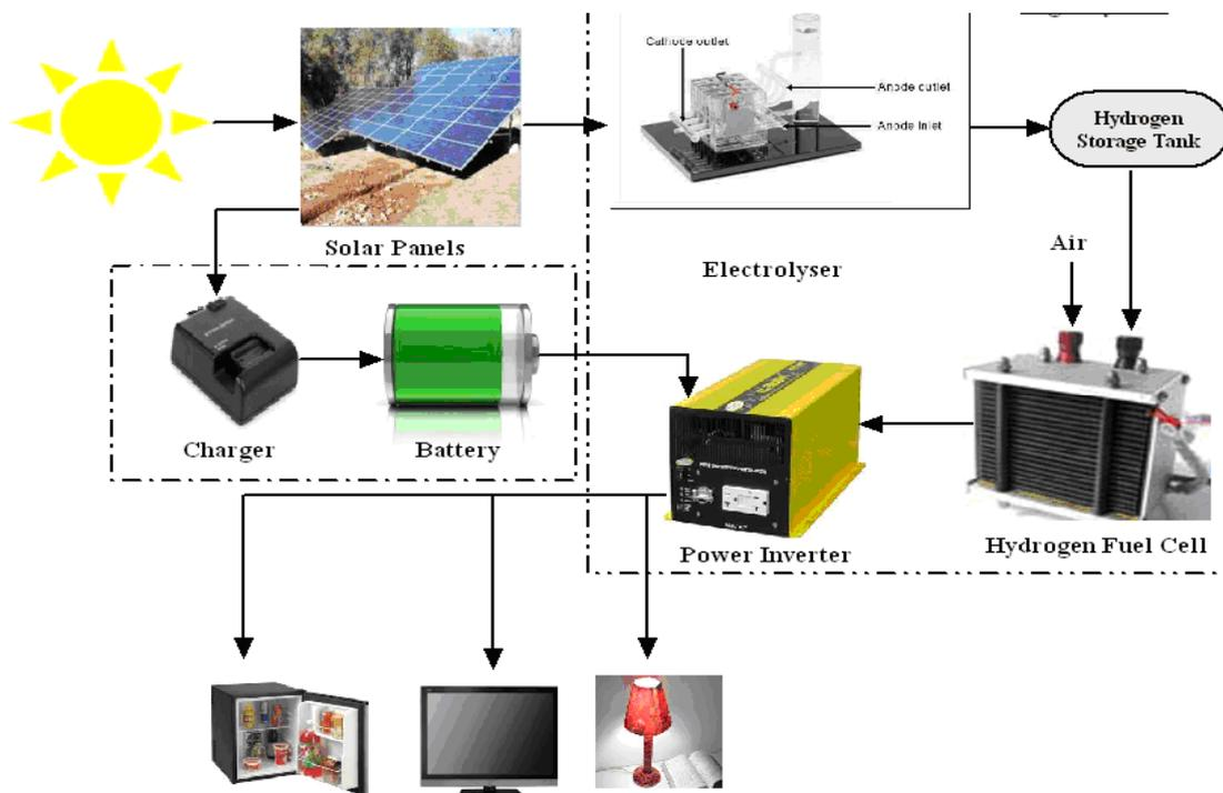
**Figure 6:** The proposed solar Hydrogen Fuel Cell system
