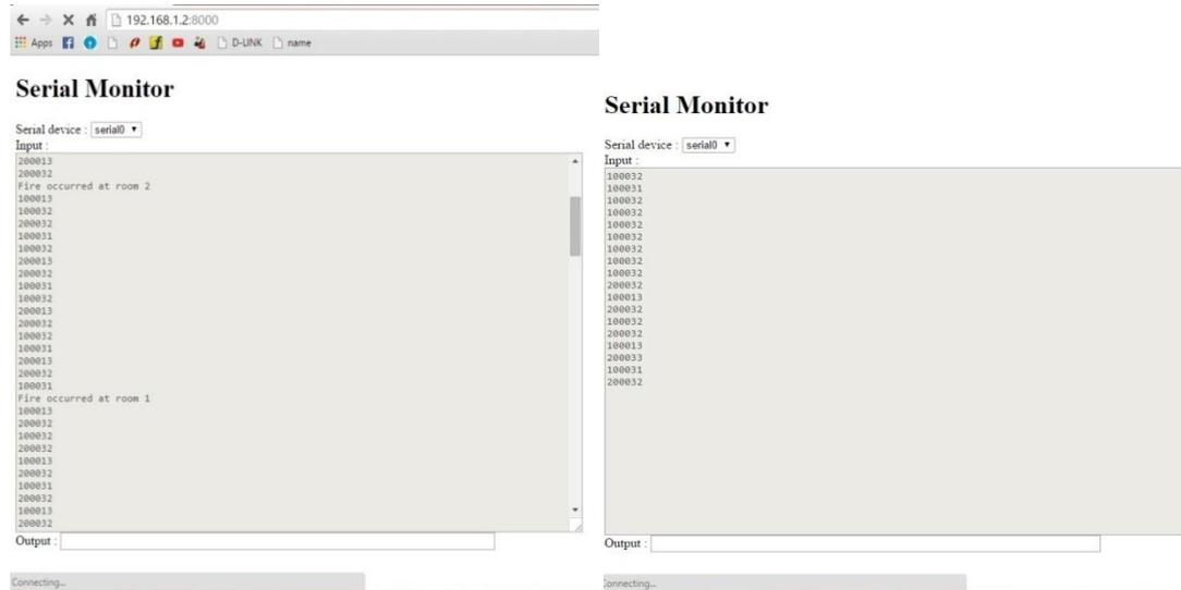
The data received from sensors is encoded, transmitted, decoded and displayed in the webpage. Here the message of fire occurrence is displayed when there is a fire in the room/environment considered.
