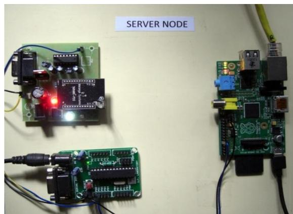
Figure 9: Server Node receiving data from client nodes
