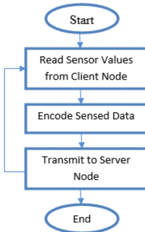
**Figure 3:** Process Flow in Client Node
