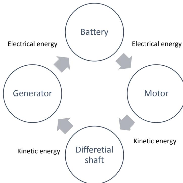
Figure 2: Block diagram of energy flow
