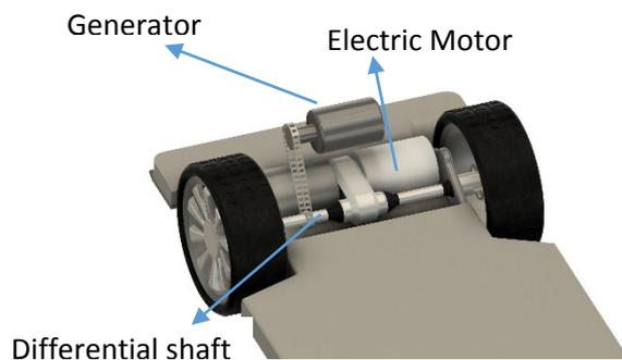
**Figure 1:-** Schematic view of arrangement of generator
