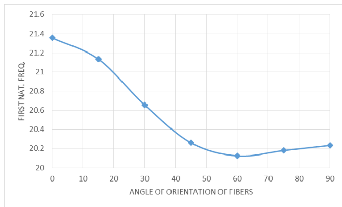
Fig. 5.1. Effect of angle of orientation of fibers on First Nat. Freq. (Hz).
