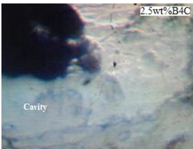
Figure 7 (c): Cavities and porosity in Al-2.5wt%B 4 C
