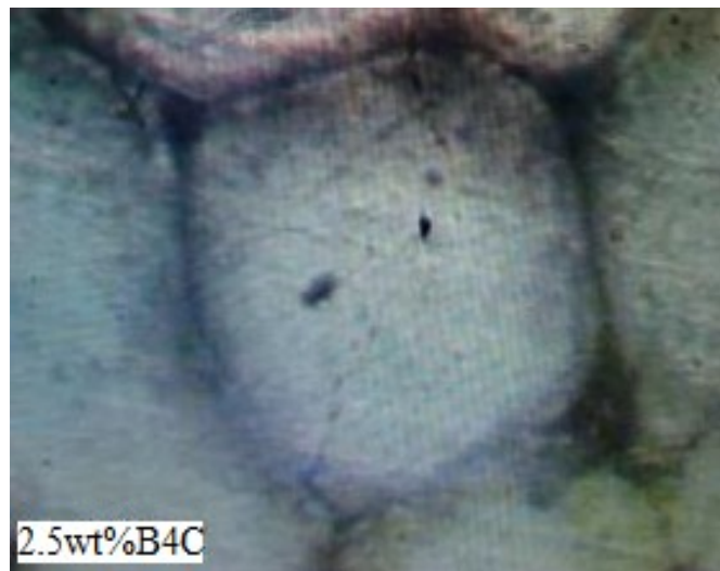
Figure 8(a): Grain size Al-2.5wt%B 4 C at 500x
