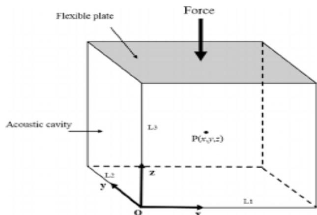
Fig.1: System Geometry
