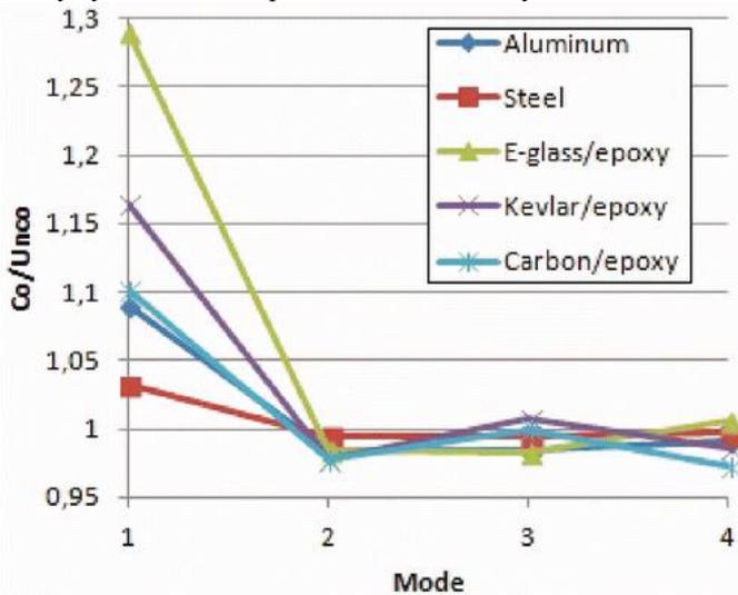
Fig.2: Comparison of the Coupled/Unco frequency ratios for the first four modes of the plates with different materials [1].
