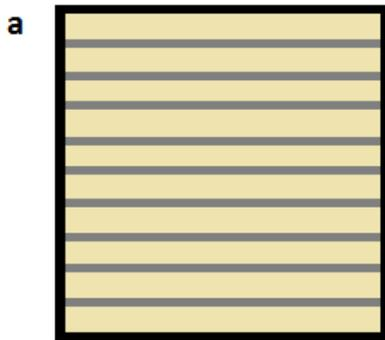
Fig.3: Composite panel at different 0° fibre orientation [31]
