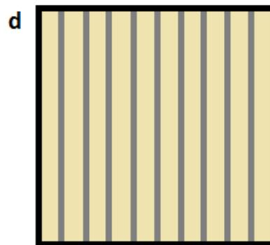
Fig.3: Composite panel at different 90° fibre orientation [31]
